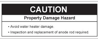
The anode rod is used to protect the tank from corrosion. Most hot water tanks are equipped with an anode rod. The submerged rod deteriorates to protect the tank. Instead of corroding the tank, water ions attack and eat away the anode rod. This does not affect the water's taste or color. The rod must be maintained to keep the tank in operating condition.
